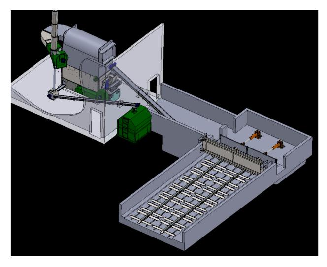
Of all the solid fuel/biomass storage technologies available we have found the reciprocating floor system to be the most adaptable, simple and low maintenance. The reciprocating or more commonly referred to as a "walking floor" is a fuel storage/handling system that allows bulk biomass fuel to transition from a storage area into the fuel feed circuit as called for by the power system it is supplying.
